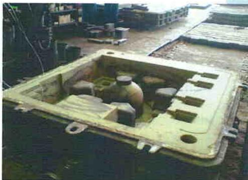
Geopol A differs from other inorganic binder systems, by the nature of the bond that is formed. Unlike Sodium Silicates, Geopol A forms an amorphous Geo-polymer, exhibiting significantly higher strengths, resulting in lower addition levels, typically 2%.
