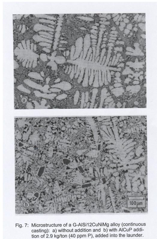
Fig. 7: Microstructure of a G-AISI12CuNiMg alloy (continuous casting): a) without addition and b) with AlCuP addition of 2.9 kg/ton (40 ppm P), added into the launder.
